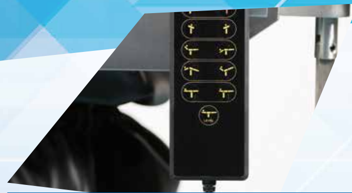
The whole operating plane can be leveled using a single button
